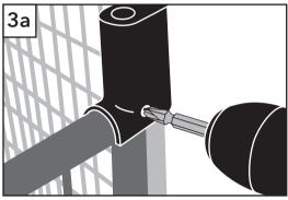
**3a**To turn your **Pet Gazebo** into a semi-permanent structure (optional), use a power drill and screw the **Self Tapping Screws** into the predrilled holes provided on the connectors for 234XX series.
