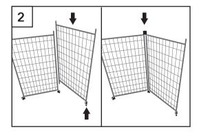
2 Place a Nylon Panel Connector on to one side of another Side Panel and insert the second Side Panel into a Nylon Panel Connector of the first Side Panel.
