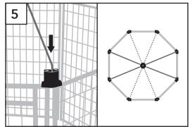
5 Insert the end of a Roof Support Arm into the larger hole of the Nylon Panel Connector.
