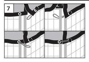
7 Using the Ball Ties provided attatch the Canopy to the posts of the kennel.
