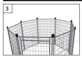
3 Repeat these steps until you have an octagonal shape. Make sure the Gate Panel and Latching Window Panel are placed where both panels can be opened from the outside.
