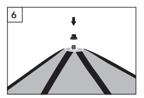
6 Make sure the Market Umbrella Canopy is oriented with the Pet Gazebo logo outward. Locate the center eyelet and line it up with the center of the Roof Support Hub.
